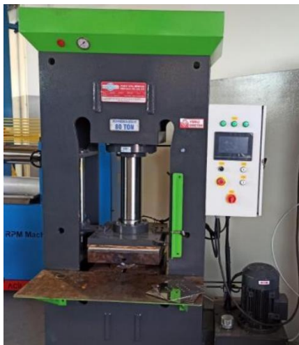
Figure 1. 80-ton hydraulic press: 4 kW power, 400mm*400mm plate, heatable up to 200 degrees, time control, PLC control panel.
