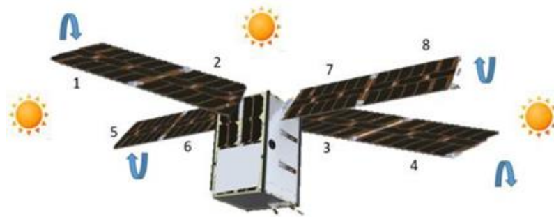
Fig. 5. Functional solar cell configuration schematic in array and panel's structure
